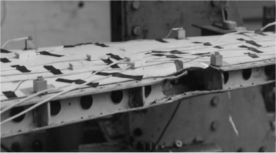
Figure 11. Structural damage on one side of the tail-plane.
